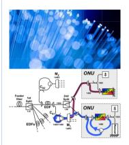
New design of the common passive power splitter used in GPON and EPON standards.
